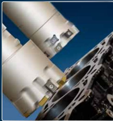
Machining of cylinder crank cases
