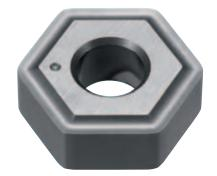
SU is designed for machining exotic materials such as Inconel. Its very sharp geometry reduces built-up-edges created while machining. The very smooth chipbreaker shape delivers chip control in sticky material and reduces crater wear.
