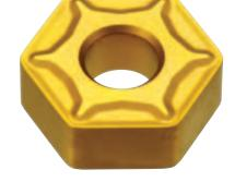
GU is designed for general machining in various materials such as steel, alloy steel and cast iron. Its 6 degree top rake angle is very secure and shows good performance in medium to roughing applications.
