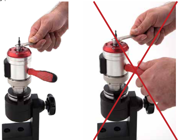
Figure 36: Tightening ER11 nut
