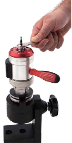
Figure 34: Loosening ER11 nut
