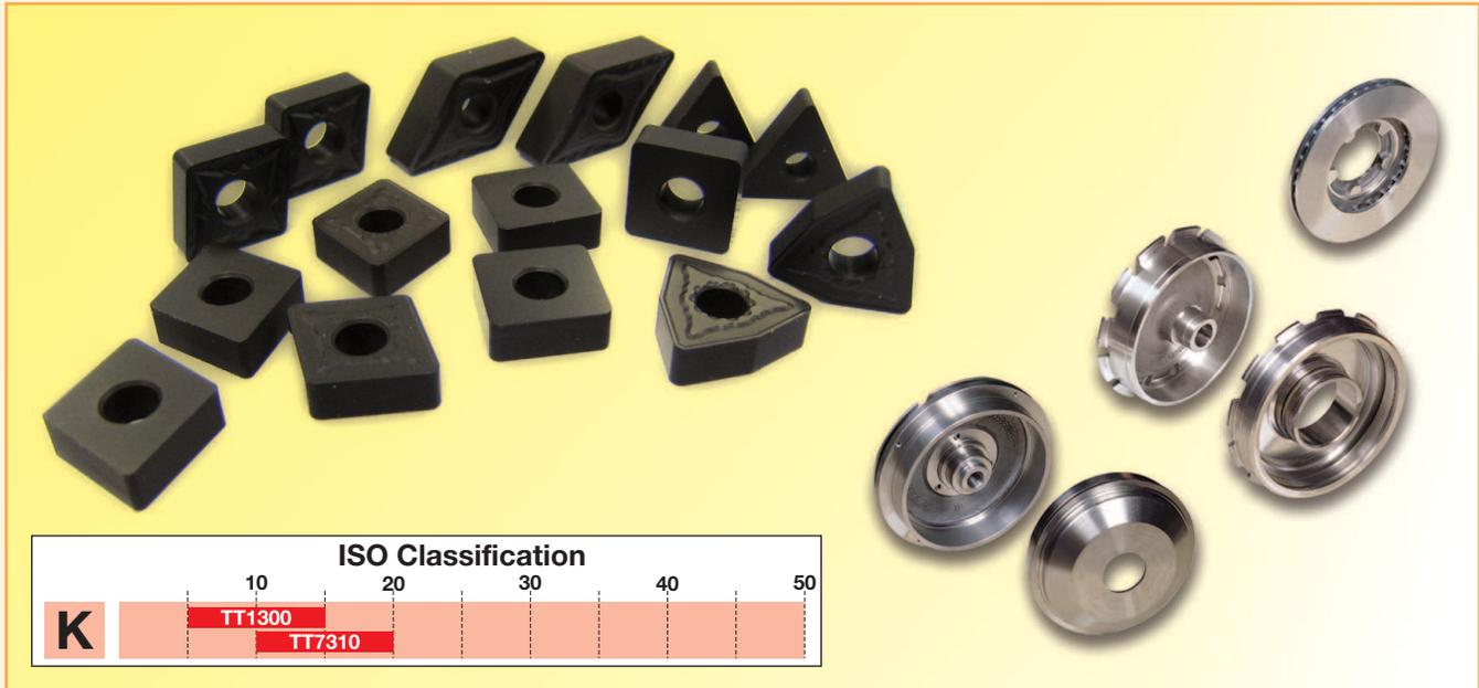
Ingersoll introduces within its TaeguLine of ISO turning inserts a new T-CAST grade, TT7310, specifically designed for cast iron applications. This new generation grade provides exceptional performance in ductile cast iron, and can also be used in gray cast iron at medium to high cutting speeds. TT7310 compliments our existing T-CAST TT1300 grade that is ideal for gray cast iron applications at very high cutting speeds.
