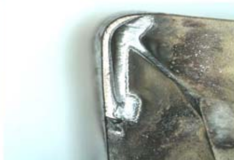
CNMG432MT TT8115 After 300 linear inches
