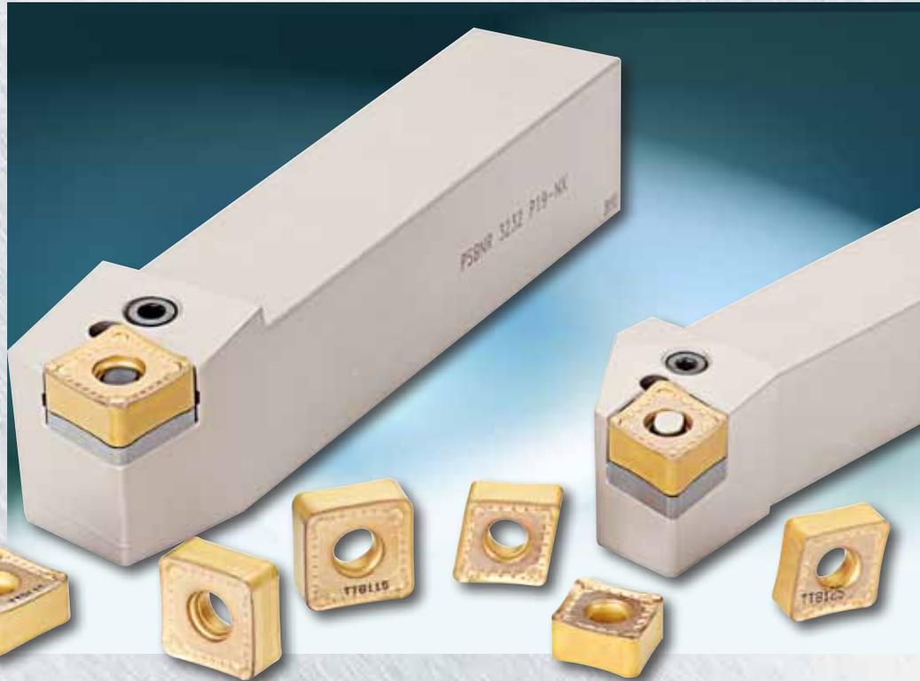
Ingersoll introduces a revolutionary new concept for general turning applications. CNMX and SNMX inserts with an HB chip breaker deliver low cutting forces and better surface finish in medium to rough machining compared to equivalent CNMG/SNMG inserts.
