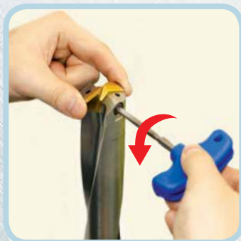
To unclamp, rotate the screw 3-5 times counter-clockwise
