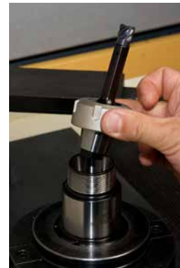
Place the nut/shank assembly into the holder
