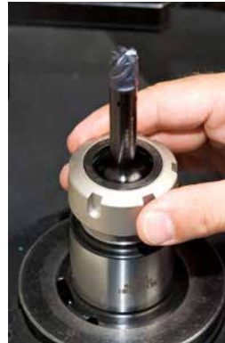
Screw the nut on the holder
