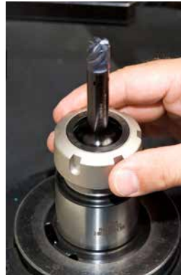
Screw the nut on the holder
