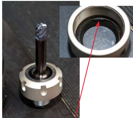
Assemble the nut with the shank by mating the Retension Tabs with the ER Groove
