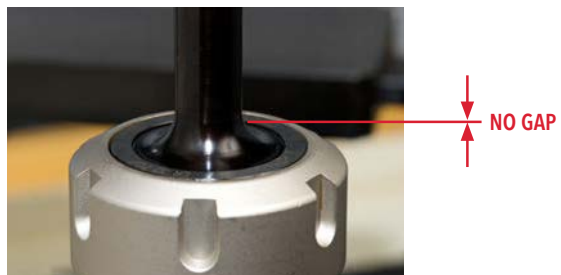
Assemble the nut with the shank by mating the Retension Tabs with the ER Groove
