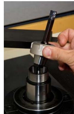
Place the nut/shank assembly into the holder
