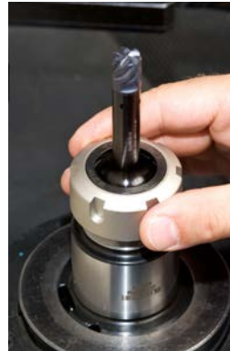
Screw the nut on the holder
