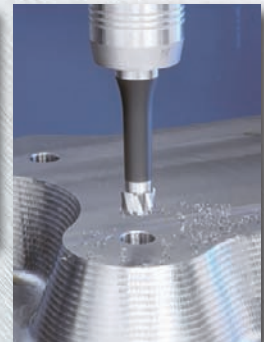
PCD tip for machining aluminum
