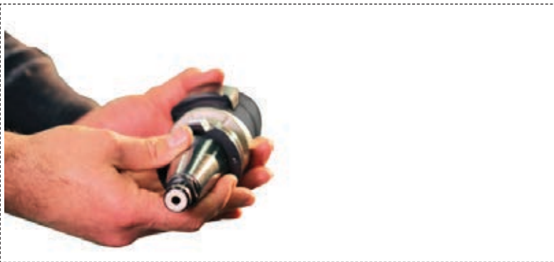
Fig. 30. Example of toolholder with a coolant-through hole
