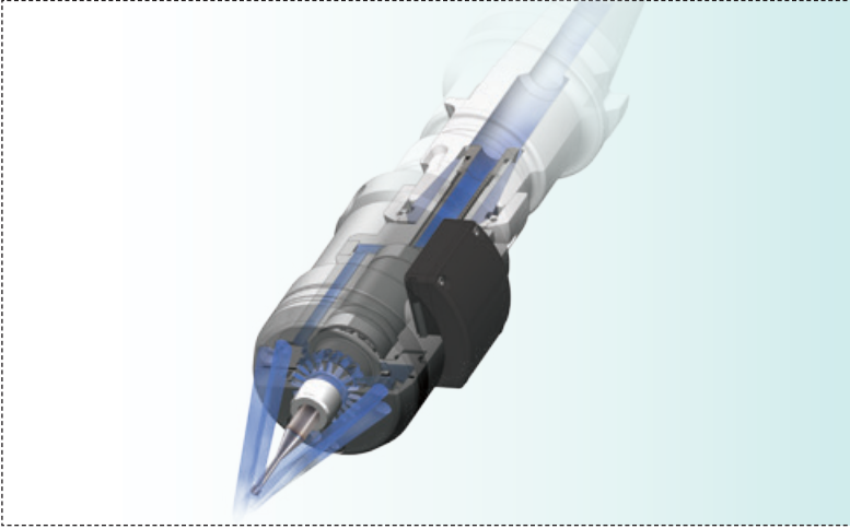
Fig. 10. Integrated coolant nozzle system
