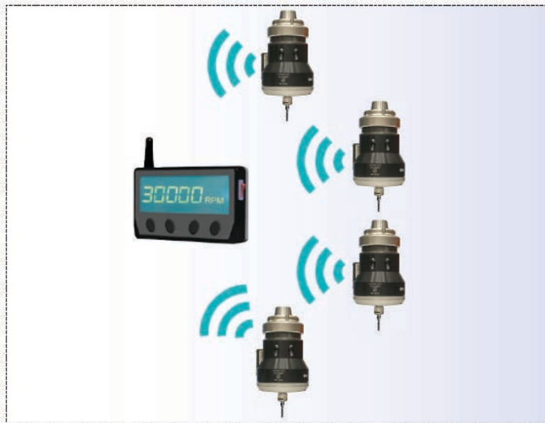
Fig. 14. Several Spindles (not working simultaneously) connected to one display
