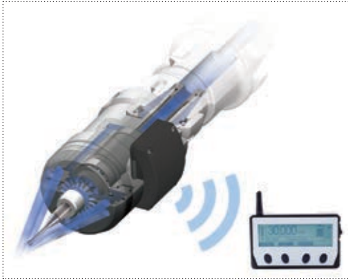
Fig. 10. Integrated coolant nozzle system
