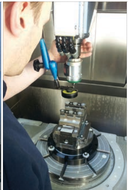
Fig. 37. Manual runout testing
