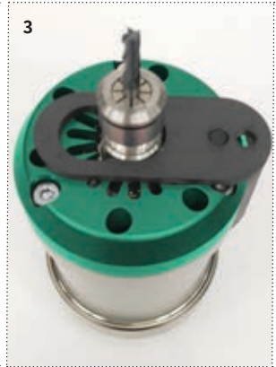
Fig. 34. Slide key into place
