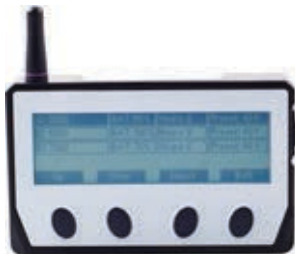
Fig. 21. Disconnection list on Multiple Signal screen
