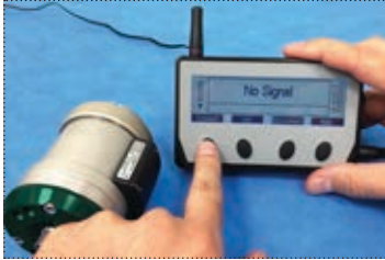
Fig. 13a. Press 'Connect' button on the display
