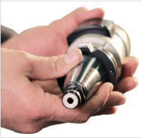
Fig. 30. Example of toolholder with a coolant-through hole
