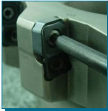
\*Tighten the insert screw completely (35in. lbs.)
