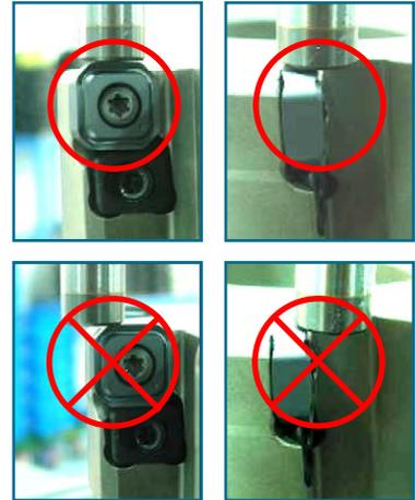
**5.1** Adjust AXIAL RUNOUT by rotating the wrench gradually until it meets the 0.005mm (.0002") range.
