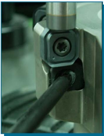
**6** RUNOUT adjustment is completed. (Do not clamp the insert screw any further once it is fixed.)
