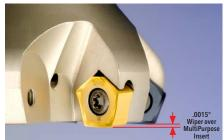
When placing one wiper insert (in one pocket), the long wiper flat is .0015" higher that the other inserts (in other pockets).
