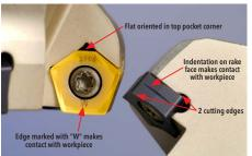
Wiper inserts have 2 indexes and should be oriented as shown above.
