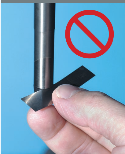
Figure 3a. Shim should NOT enter intersection
