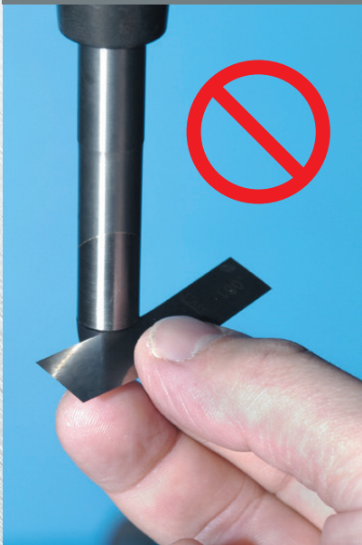
Figure 3a. Shim should NOT enter intersection
