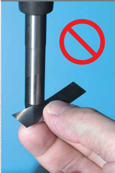
Figure 3a. Shim should NOT enter intersection
