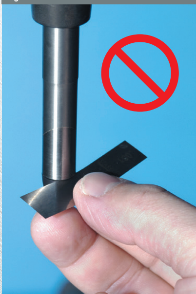
Figure 3a. Shim should NOT enter intersection
