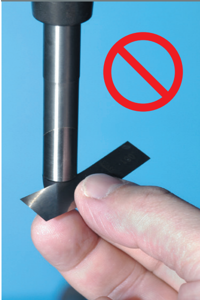
Figure 3a. Shim should NOT enter intersection
