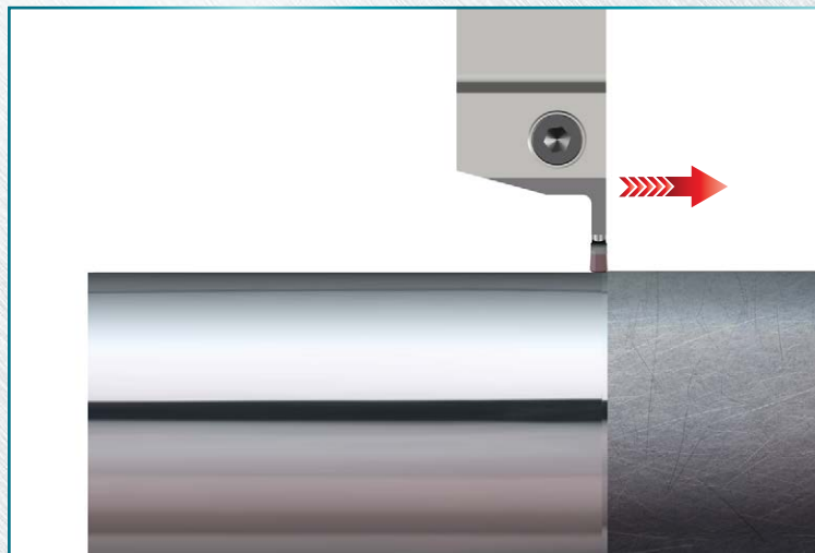
High feed turning with excellent surface finish
