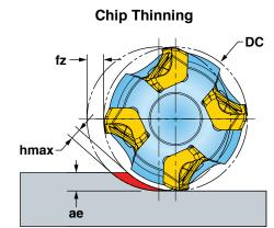
\* When ae is less than 25% DC, recommend use of Chip Thinning Calculator to ensure hmax is in fz range.
