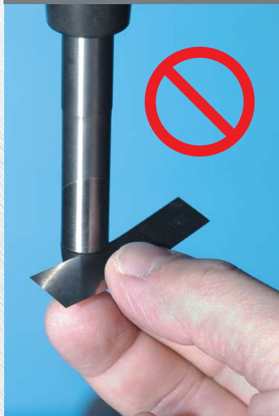
Figure 3a. Shim should NOT enter intersection
