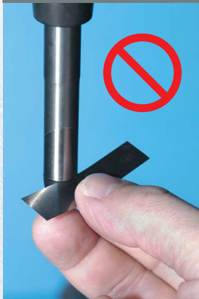
Figure 3a. Shim should NOT enter intersection
