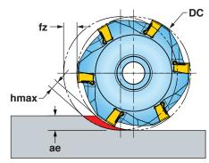
\* When ae is less than 25% DC, recommend use of Chip Thinning Calculator to ensure hmax falls within fz range.
