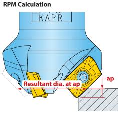
Calculation is to be made using the resultant diameter at ap.
