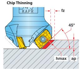
Chip Thinning Calculator is recommended to ensure hmax falls within fz range.
