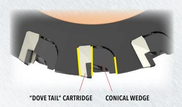
The precise height is guaranteed from the regulation of the adjusting wedge, that is placed below the cartridges. This product line also offers different cutting edge geometries to satisfy the customers requirements.
