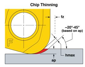
\* Chip Thinning Calculator is recommended to ensure hmax is within range.
