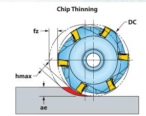
\* Chip Thinning Calculator is recommended to ensure hmax is within fz range.
