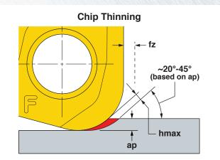
\* Chip Thinning Calculator is recommended to ensure hmax is within range.
