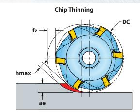
\* Chip Thinning Calculator is recommended to ensure hmax is within fz range.
