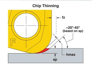
\* Chip Thinning Calculator is recommended to ensure hmax is within range.
