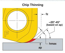
\* Chip Thinning Calculator is recommended to ensure hmax is within range.
