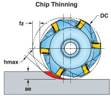
\* When ae is less than 25% DC, recommend use of Chip Thinning Calculator to ensure hmax falls within fz range.
