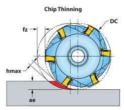
$^{\ast}\,$  Chip Thinning Calculator is recommended to ensure hmax is within fz range.
