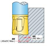
When spotfacing (full diameter), depth of cut (ap) should not exceed .35 x DC.
