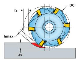
\* Chip Thinning Calculator is recommended to ensure hmax falls within fz range.
