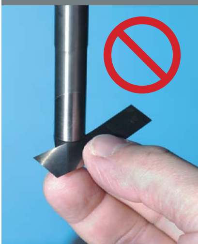
Figure 3a. Shim should NOT enter intersection
