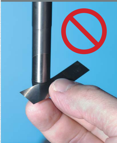
Figure 3a. Shim should NOT enter intersection
