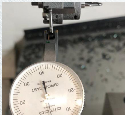
4 Use a dial indicator to align the spindle housing on the ground edge.
