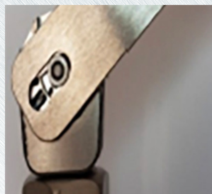
2 Lock the shaft using the dedicated key as shown in the picture, and screw the collet in position.
