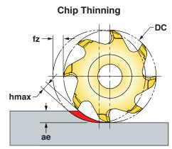
\* When ae is less than 25% DC, recommend use of Chip Thinning Calculator to ensure hmax is within fz range.
