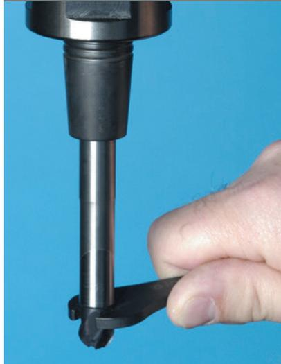
Figure 3a. Shim should NOT enter intersection
