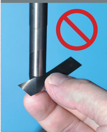
Figure 3a. Shim should NOT enter intersection
