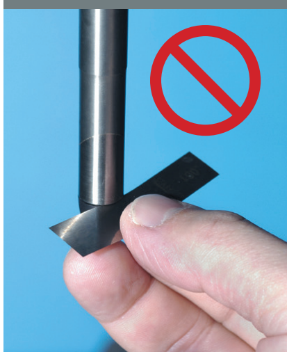
Figure 3a. Shim should NOT enter intersection
