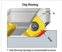
\* Chip Thinning Calculator is recommended to ensure hmax is greater than .003"
