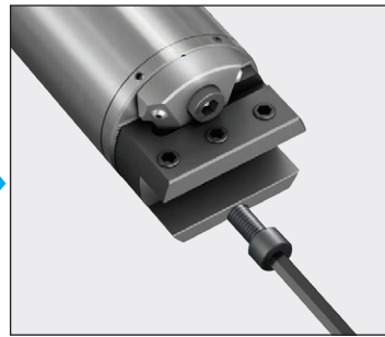
2. After sliding the adapter into the boring bar, tighten the clamp screw.
