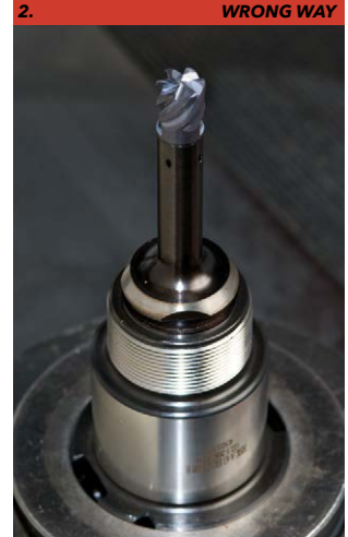
2. Place the integral ER collet into the collet chuck.
