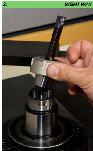
3. Place the nut/shank assembly into the holder and secure the nut.
