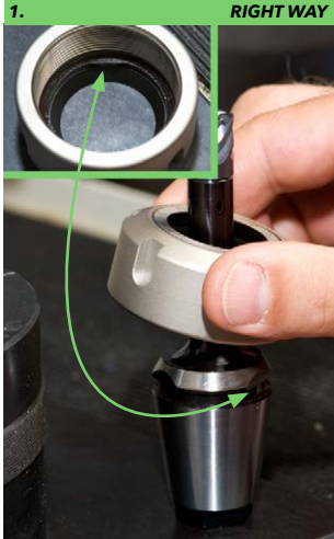
1. Place the nut on the integral ER collet. Assemble the nut with the shank by mating the retention tabs with the ER groove.
