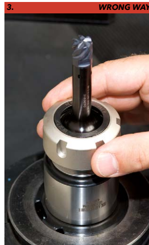
3. Screw the nut on the holder.
