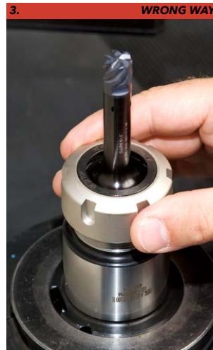
3. Screw the nut on the holder.
