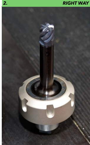
2. The nut/shank assembly is shown ready for installation.
