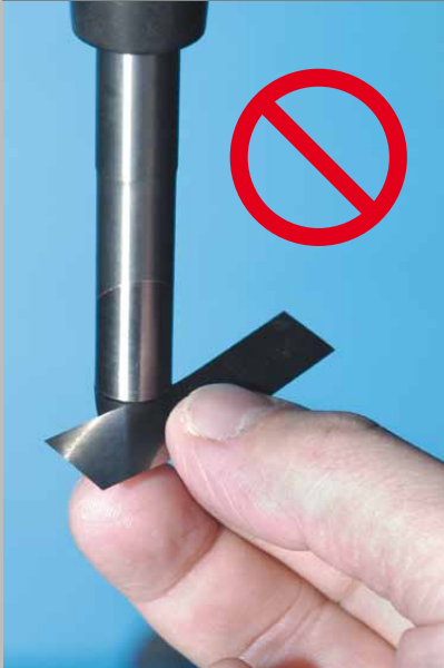
Figure 3a. Shim should NOT enter intersection
