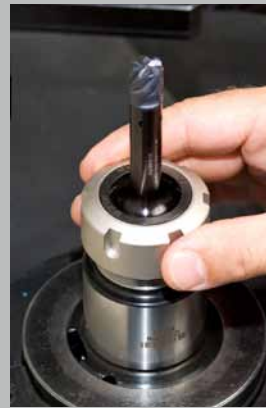
Screw the nut on the holder
