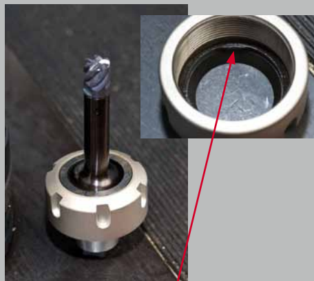
Assemble the nut with the shank by mating the Retention Tabs with the ER Groove
