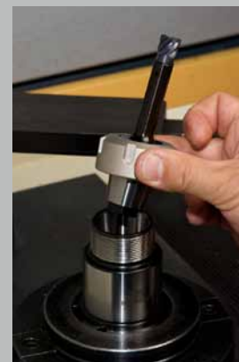
Place the nut/shank assembly into the holder
